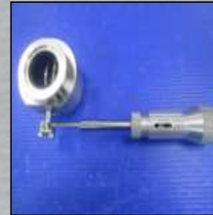
To use “扭力扳手” to fix coupling. (14 kg-cm)
