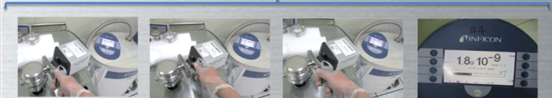
Vacuum test by He detector
